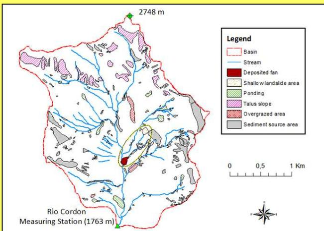
Sediment sources areas: cliffs, shallow landslides, eroding stream banks and small debris flow channels
